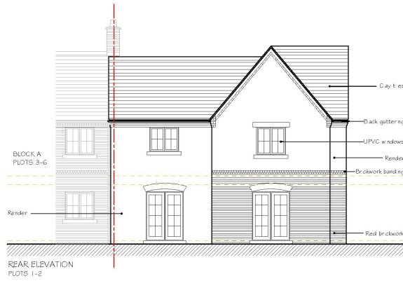
0 10m HOUSE TYPE C_Elevations_2B 4P_Semi-Detached (1:100)
